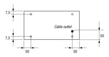
Type "C" Frame-plate flush with the bumper and with M6 stud bolts, 30 mm long, for fastening to the inside of the machine via bolts.
