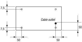
N.B. For bumpers longer than 500 mm, other additional fastening holes will be drilled (centre distance from one hole and another  $\leq$  500 mm.
