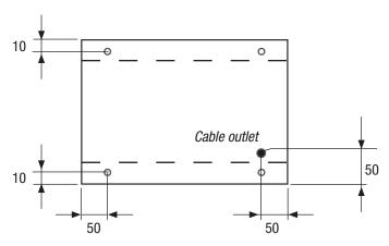
**Type "B"** Frame-plate flush with the bumper and with threaded holes (specify when ordering) for fastening to the inside of the machine via screws.
